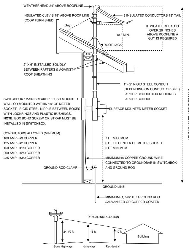
MINIMUM 12 FT. ABOVE GROUND TO INSULATED CLEVIS (12' 6" TO WEATHERHEAD)
